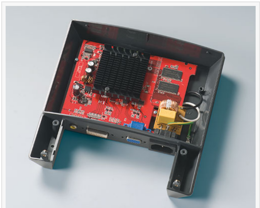
NET-BOX with has plenty of space for the PCBs
