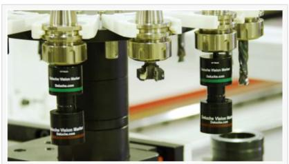
The DeLuche Vision Marking Tool plugs directly into any tool holder with a 1/4" shank, and works with popular cabinet cutting software.
