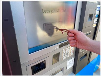
A capacitive screen is made from layers of glass and plastic that are coated with a conductor material like indium tin oxide or copper. CuRVE's Copper Alloy completes the circuit when it contacts a screen.
