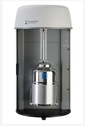
Micromeritics TriStar II Plus 3030 Surface Area and Porosity Analyzer
