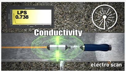
Low Voltage Conductivity provides unbiased, unambiguous, and uncontested water leak locations and an estimated liters per second for each defect, with readings generally recorded during pull back when the Hydrochute is collapsed.
