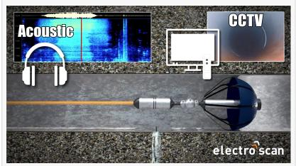
Traditional acoustic sensor provides general sound patterns, while CCTV cameras are used as navigational aid and to document obstructions and customer connections, traversing inside a pipe propelled by an innovative Hydrochute.
