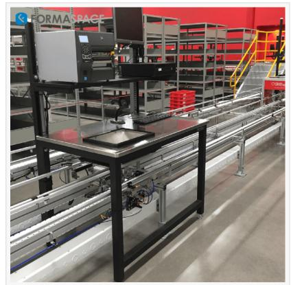
Here is a stainless steel top we built for a large pharma supplier that features a stainless steel top workbench with a built-in cutout for custom scale.
