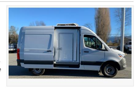
refrigeration lineup, the Pluto Dual is a fully-battery powered refrigeration unit available for delivery vehicles. It can run for up to 10 hours solely on battery power on all electric installs, though it also has the ability to be charged via diesel or gasoline engines.
