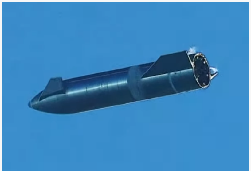
Starship prototype SN8 during its successful "belly flop" gliding maneuver. Credit: SpaceX
