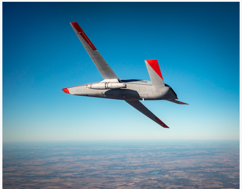
An MQ-25 flies with a Cobham aerial refueling store. Credit: Boeing
