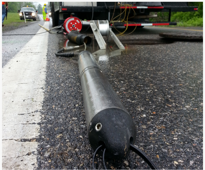
Electro Scan ruggedized machine-intelligent pipeline assessment probe.
