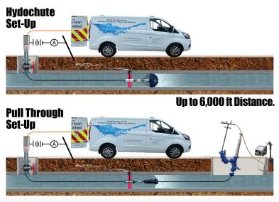
Electro Scan can find & measure leaks either with or without pressure, ranging from ZERO to 175 psi.
