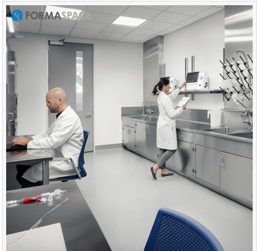
Formaspace manufactured this impressive stainless steel lab for analyzing blood at a medical device manufacturer. The bench is exceptionally long, a full 24' feet of seamless stainless steel work surface with multiple built-in wet sinks.
