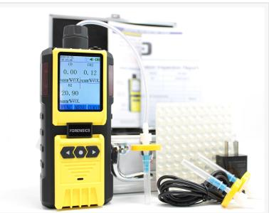
Headspace Analyzer Carbon Monoxide, Carbon Dioxide and Oxygen
