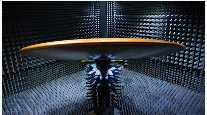
NSS ESA Antenna in Test Chamber
