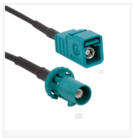
performance industry standard FAKRA connectors that are mechanically keyed and color coded to avoid mismating during the installation process. The FAKRA assemblies support frequencies through 3 GHz which allows them to meet the requirements of automotive applications such as 360-degree cameras, remote start and Advanced Driver Assistance Systems (ADAS).
