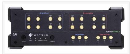
The hybridNETBOX model DN2.825-04 provides four AWG channels that can output waveforms at rates up to 625 MS/s with 16-bit resolution, along with four digitizer channels that can each sample signals at 500 MS/s with 14-bit resolution.
