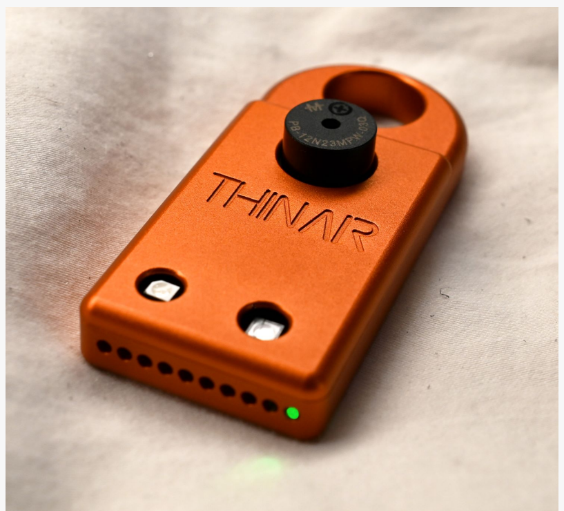
Geiger UVc measures strength and dose of UVc source
