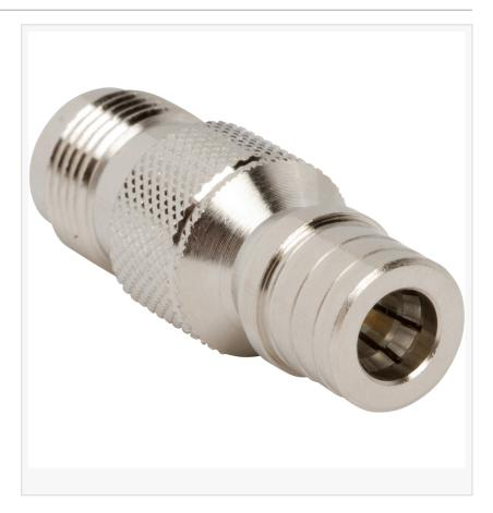
QMA adapters offer reliable low loss performance up to 18 GHz with high power handling. They are designed with brass bodies that are either gold or white bronze plated depending on the specific configuration. Multiple configurations are available to support a wide range of application needs and improve capabilities of existing systems.
