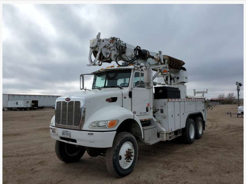
2010 Peterbilt 348 Digger Derrick Truck
