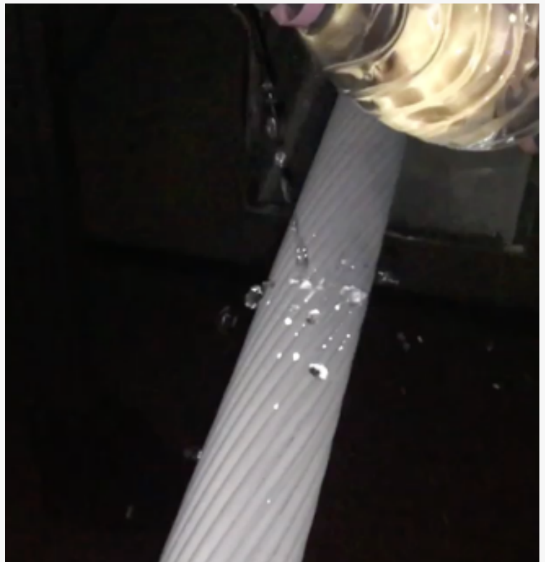
Nanto Paint® Durable Superhydrophobic coating effect on electric wire cable 2018
