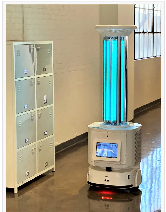
Black-I Environmental PureTech autonomous disinfectant robot at work in Rochester, NY, hospital
