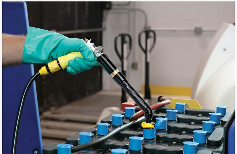
Using a Gun-X to water a lead acid battery
