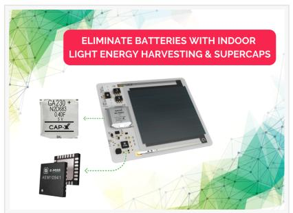
Epishine, CAP-XX, and e-peas created an indoor light energy harvesting solution to power small, lowpower, battery-free devices that are normally powered by batteries.
