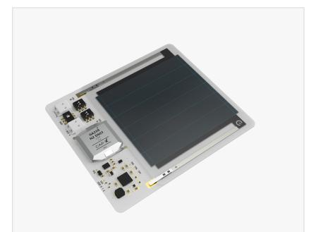
The compact evaluation module (81 x 71.5 x 3.8mm) contains everything needed for manufacturers to test if the solution will generate enough energy to power their devices without a battery.
