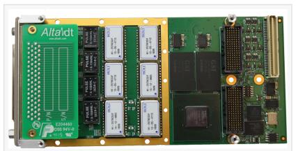
XMC-1553 - The Industry's Most Advanced 1553 Interface for VME, VPX, cPCI, PXI Systems
