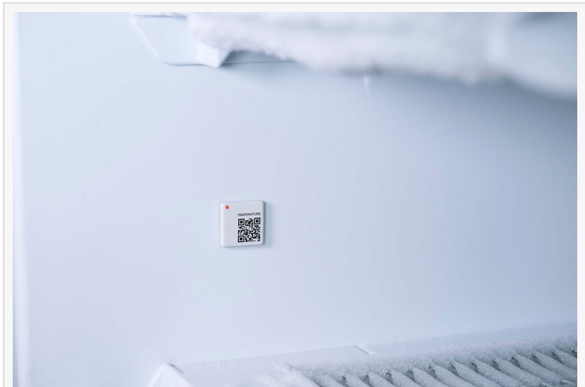
The QR code is a Model 2 type QR code and contains the sensor ID
