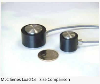
stainless steel. The sensing element incorporates bonded foil strain g ages to produce a full scale output of 2mV/V. Accuracies are Nonlinearity .25%, Hysteresis .25%, and Nonrepeatability 0.1% or better. Load cells are supplied with a Certificate of Calibration traceable to N.I.S.T.
