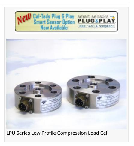
Nonlinearity 0.1%, Hysteresis 0.1%, and Nonrepeatablility 0.05% or better. They are sealed for protection against most industrial environments and are supplied with a <u>Load Cell Calibration</u> Certificate traceable to N.I.S.T.
