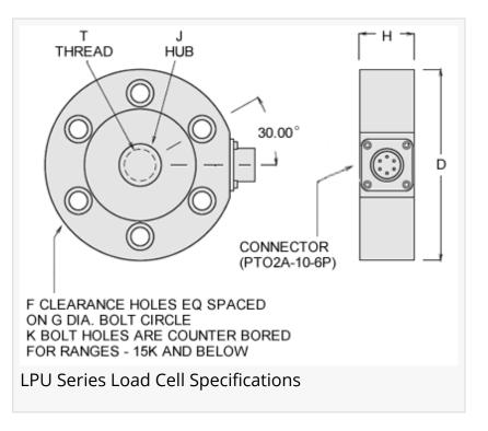
to close tolerances. The strain gauges are electrically connected to form a balanced Wheatstone bridge and additional compensation resistors are added to the circuit for maintaining the accuracy of the bridge over a wide temperature range.
