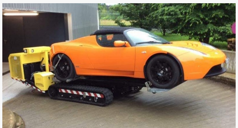
TowTract carrying a disabled Tesla out of a 6' parking garage because a truck is too tall to get in.
