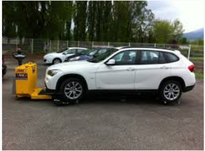
CarTrack carrying an all-wheel-drive vehicle without keys.
