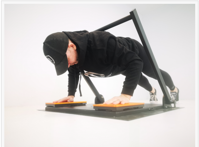
Isophit inventor Brad Thorpe demonstrates and measures an isometric push on the Isophit M.S.K with Kinvent's KForce Plates.
