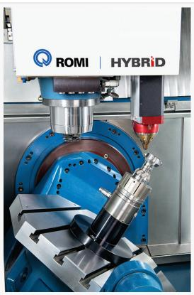
Simultaneous Machining on all Five Axes
