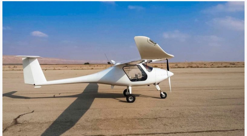
ALBATROSS is based on Pipistrel Sinus Aircraft and designed for long-term flights in conditions of high turbulence and overload.
