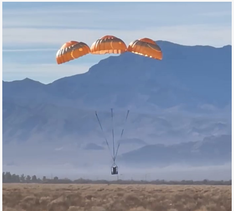
Testing of ASR recovery parachute system for eFlyer 2. Photo credit: Aviation Safety Resources, Inc.
