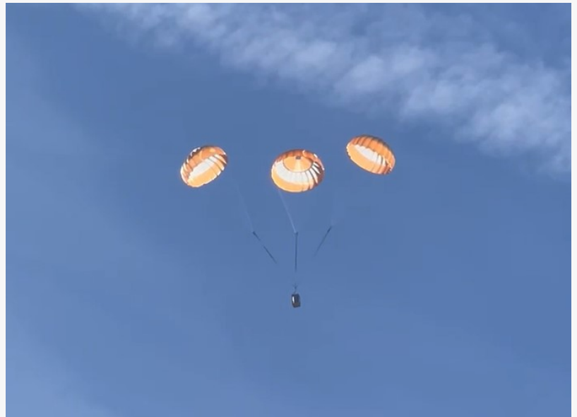
Testing of ASR recovery parachute system for eFlyer 2. Photo credit: Aviation Safety Resources, Inc.
