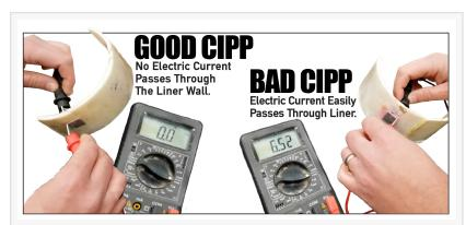
Low voltage conductivity allows utilities to automatically identify location and severity of defects in Cured-In-Place Pipe (CIPP) and other trenchless rehabilitation.
