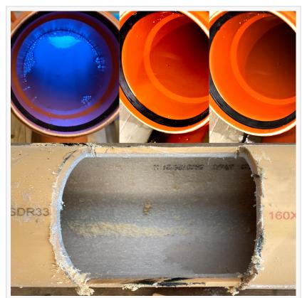
Light-Emitting Diode (LED) Cured-In-Place Pipe (CIPP) has struggled to pass leak detection tests with owners and contractors looking for precise locations and severity of leaks with Electro Scan technology.
