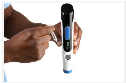
Portal Instruments' handheld connected needle-free jet injector uses ultra-power-dense CAP-XX supercaps to deliver hundreds of watts of power to drive its high-speed, concentrated injection.
