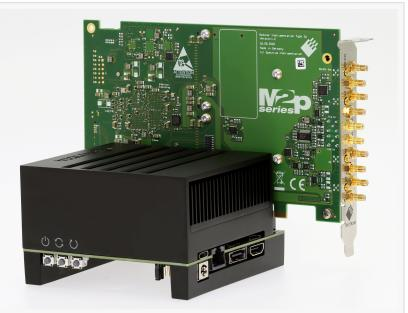
NVIDIA Jetson with a M2p.5968 digitizer card from Spectrum: This small but powerful combination is able to sample eight signals in parallel with 125 MS/s.
