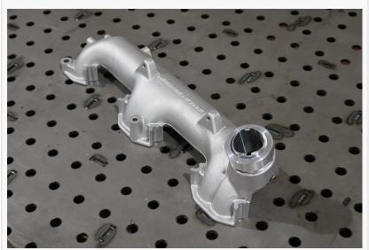
The adapter fits easily inside the om617 intake and provides a solid intercooler connection point.
