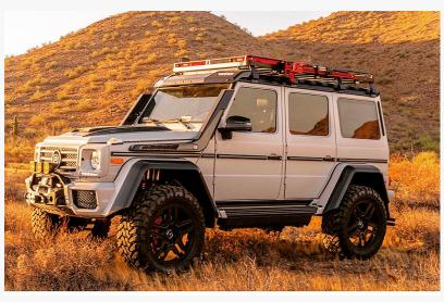
G550 Squared Edition equipped with a Bi-turbo 4.0L V-8 engine, 620 HP and 590 lb-ft of torque. This specimen boasts luxury upgrades such as full rooftop rack, off-road Rotopax fuel cans, Hi-Lift Jack Shovel, auxiliary overhead front lights, side and rear-facing front mounted amber hi power off-road lights, and a Warn 10,000 lb. Winch with synthetic cable. The off-road potential
