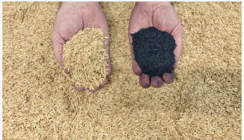
Glanris hybrid green water filtration media made from rice hulls
