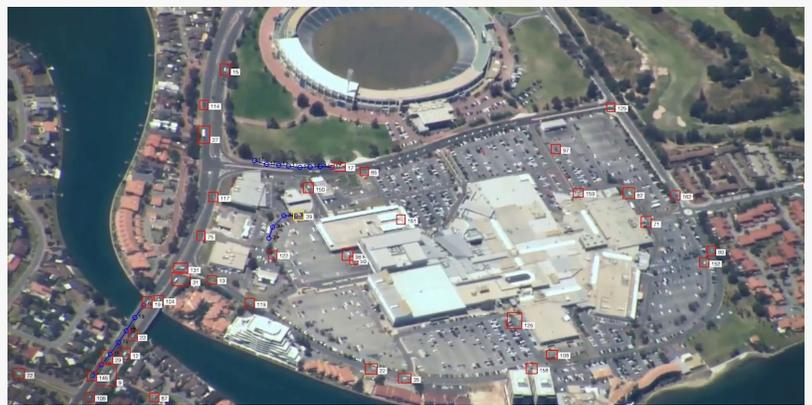
This video still frame demonstrates how Sentient Kestrel can detect and track multiple targets based on motion – reducing operator fatigue and identifying objects that might otherwise be too small for operators to see.
