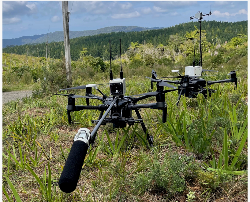
Dotterel two-way audio drone perched ready for bush emergency rescue
