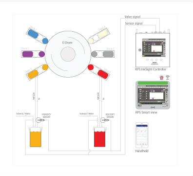
Real-time ink viscosity control is achieved by viscosity sensors & correction valves on each print deck. Ink viscosity is controlled so accurately that it ensures highly consistent color density over complete print.
