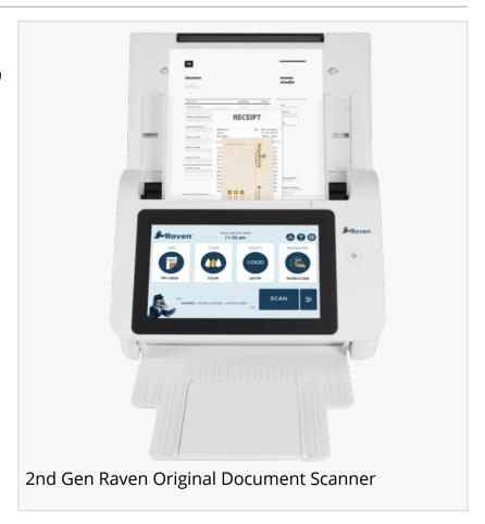
Scanner comes with a larger 8 inch LCD touch screen display, the largest in the category. The scanner automatically detects and removes blank pages, automatically orients / rotates pages and has ultrasonic multifeed and paper jam detection. "The hardware has been completely redesigned to improve functionality, usability and efficiency" said Raven CEO, Stefan Diasti.
