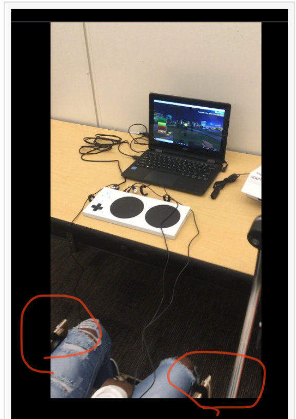
Custom controls — Our game (PC version), with Xbox Adaptive Controller, and switches attached to student's wheelchair.
