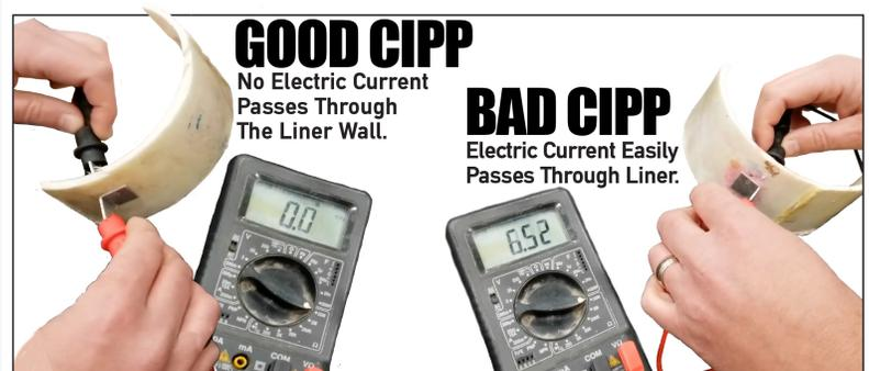
Low voltage conductivity allows utilities to automatically identify location and severity of defects in Cured-In-Place Pipe (CIPP) and other trenchless rehabilitation.
