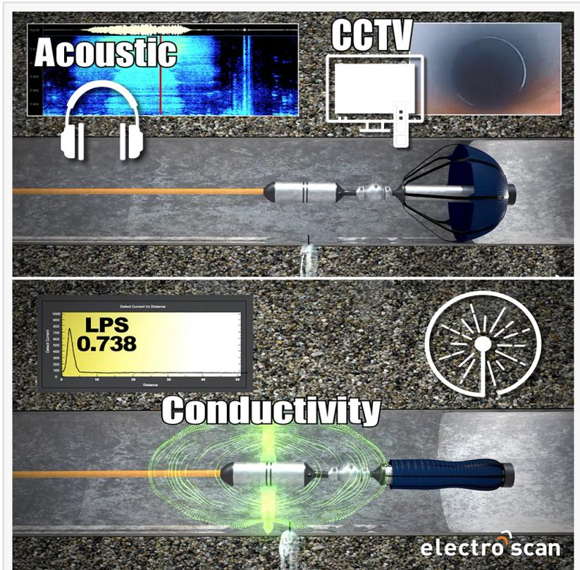
Multi-sensor probe combines Acoustic (legacy listening), CCTV (visual navigation), and Conductivity (pinpoint leak location), in a single in-pipe tethered platform.
