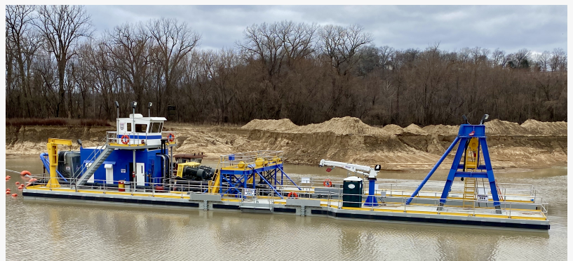
Side view of the Winter Bros new electric Chain-Ladder dredge designed and built by Custom Dredge Works
