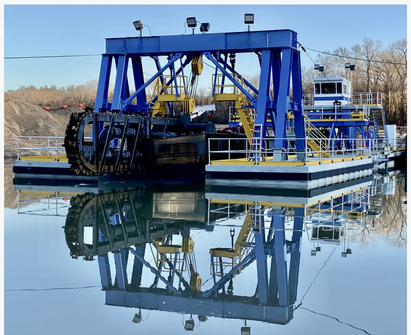
Front view of a 14" Electric Chain-Ladder Cutter Suction Dredge owned by Winter Bros. Material
