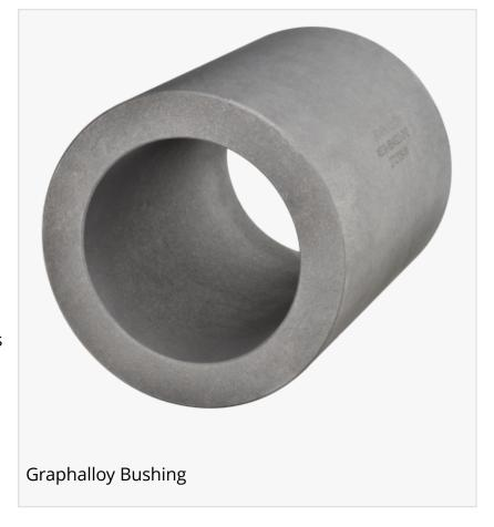
screw compressor in dihydrogen gas service. It is a high speed, low load application for the bushings. They had originally tried aluminum bushings, which failed, then plain bronze bushings, which also failed. They then tried Graphalloy Bushings, which have been successful in this application.
