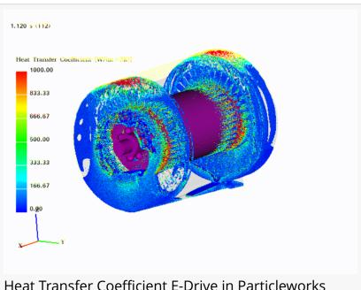
Heat Transfer Coefficient E-Drive in Particleworks simulation
