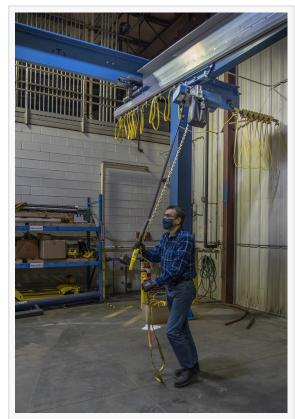
Hybrid Cranes utilize the strength and longevity of patented track with the light weight advantages of Gorbel®'s aluminum enclosed track bridges.
