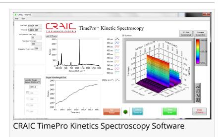
used with CRAIC Technology's microspectrophotometers and their controlling Lambdafire ™ software. CRAIC TimePro™ allows the user to monitor changes in the spectra over time. The most unique feature is that this software will allow users to measure the time dependant changes in full UV-visible-NIR range reflectance, absorbance and even emission spectra of microscopic samples. This will provide a unique and valuable tool for everything from chemistry to biological research.
