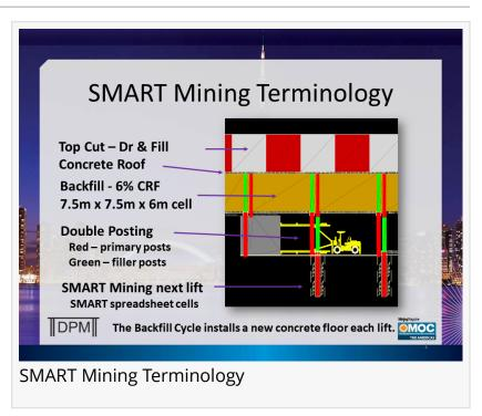
of 7.5m x 7.5m x 6m high containing ~1,000t of ore. See Image 13 for SMART details.
